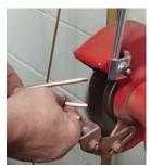
Use wire wheel to remove burrs from the cut end.
