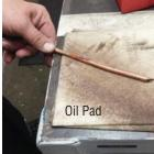
of oil to the outside surface of the water tube to facilitate installation in the adapter.
