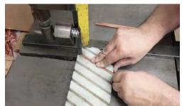
4. Cut the non-flared water tube end on an angle to specifications or as shown on the print. If available, an angle fixture is recommended; otherwise, use appropriate measures to ensure accuracy.
