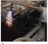
**6.** Solder the rear insert on the tube (if required). For bent adapters, soften the tube by heating to a cherry red color and quenching it in water.
