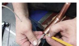
2. Remove the old water tube completely and ensure that the through hole is clear. Next, insert a flexible nylon rod through the adapter to determine the overall length; add 1.5" to this length to determine the required overall length of the water tube.
