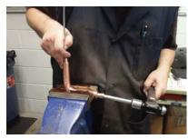
9. Continue to lightly tap the end of the water tube to push it through the adapter until it comes up to the end of the taper. Remove the flexible plastic rod.
