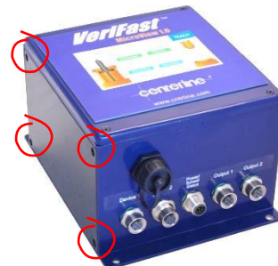
Figure 7 – Accessing the Signal Conditioner
